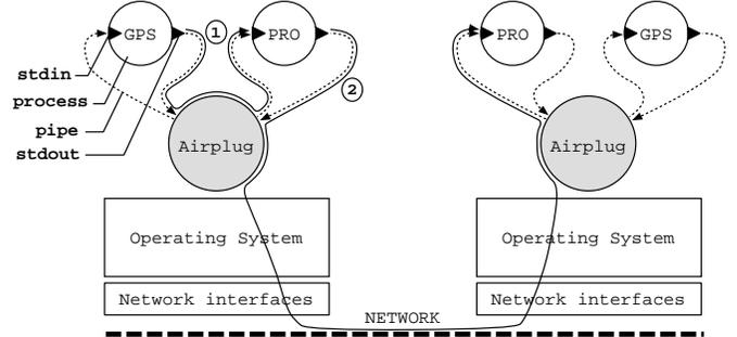
Fig. 1. Airplug architecture, intra- (1) and inter- (2) vehicle communications.
