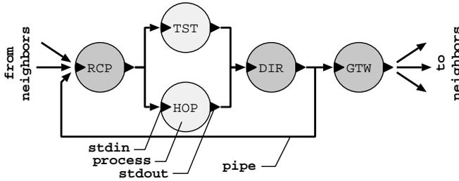
Fig. 2. Two applications (TST and HOP) in an emulated vehicle.
