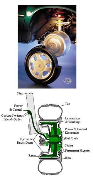
Fig. 13. In-wheel PM brushless motor layout [TM4].
