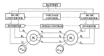
Fig. 10. Doubly fed differential drive layout [24].
