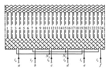
Fig. 7. Inverter-fed six-phase pole-changing IM drive [21].
