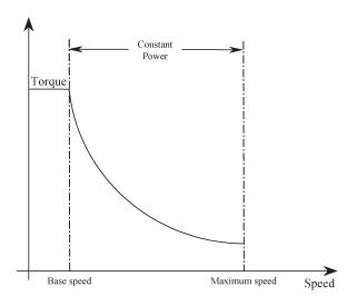
Fig. 14. Typical torque-speed characteristic of an SRM.
