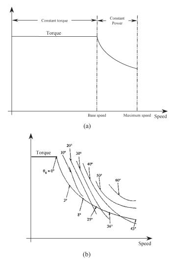
Fig. 12. Torque-speed characteristic of a PM brushless drive. (a) Typical characteristic. (b) With conduction-angle control.
