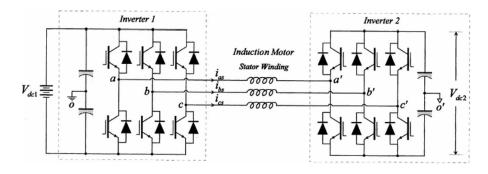
Fig. 9. Dual inverter system [23].
