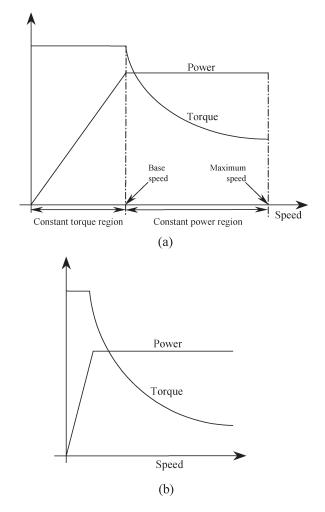
Fig. 3. HEV typical characteristics. (a) Electric traction. (b) Tractive effort versus the speed.
