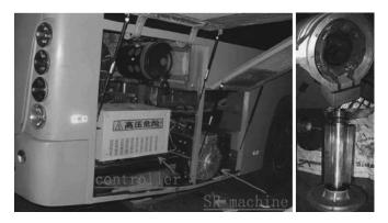
Fig. 16. A 50-kW SRM in an experimental HEV bus [31].
