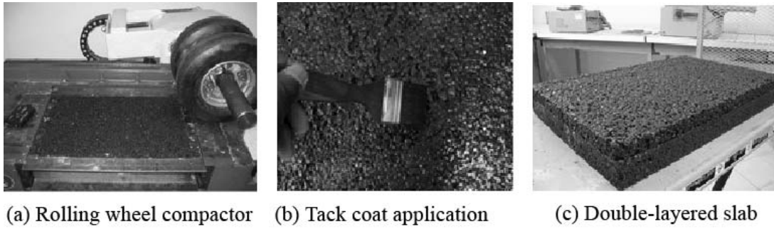
Fig. 4. Laboratory manufacturing process for a double-layered slab specimen
