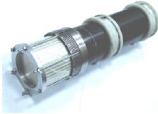
Figure 4. Photograph of the projectile/specimen system
