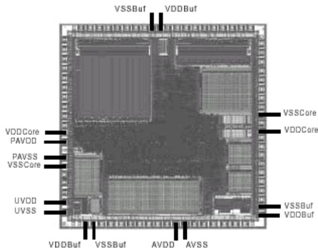
Figure 1: VDD/ VSS network of the microcontroller
