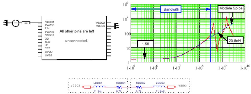
Figure 5: Measurement and model for VDDC1 and VDDC2 configuration
