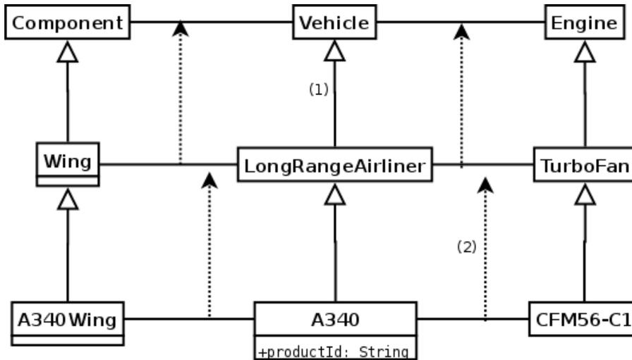
Figure 1. A metamodel of an aircraft company
