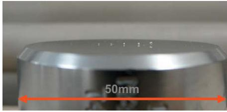
Fig. 9. Solder balls on compression die.
