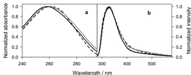
**Figure 1.** Normalized steady-state absorption (a) and fluorescence (b) spectra of DNA in pure water (grey) and in phosphate buffer (black). Excitation wavelength: 267 nm. The spectra of the stoichiometric mixture of monomers (58% of dAMP and TMP, 42% of dGMP and dCMP) in water are shown in dashes.
