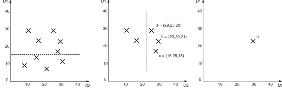
**Figure 1. A set of vectors in a three dimensional space  $D1 \times D2 \times D3$ , and the three iterations of the  $\alpha$ -trimmed lexicographical maximum computation with  $\alpha = 0.5$  (left to right). According to the proposed approach, the maximum will be the greatest, with respect to the third dimension, of the remaining three vectors.**
