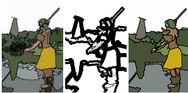
Fig. 7. From left to right, the segmentation result using the jump connection algorithm [11], the marker image and the final marker based watershed result.
