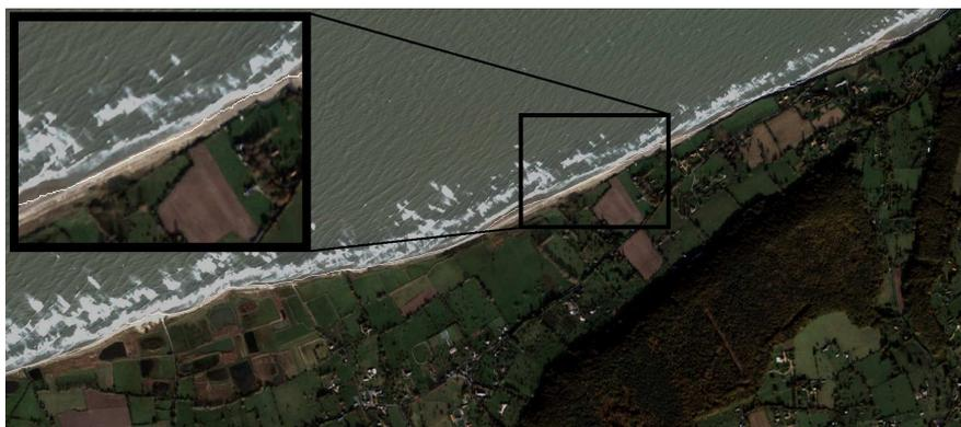
**Fig. 4.** Coastline extraction on Normandy coast QuickBird image at resolution of 2.4m per pixel ((c)Digitalglobe)
