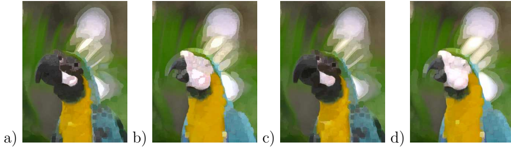
Fig. 7. The erosion and dilation results of a part of the macaws image (figure 10a) with a square shaped SE of size 9 \times 9 pixels, using \alpha -modulus lexicographical ordering (5) (a,b) and the proposed quantisation based lexicographical ordering (8) along with the priority distribution illustrated in figure 6a and both with \alpha = 50 (c,d).
