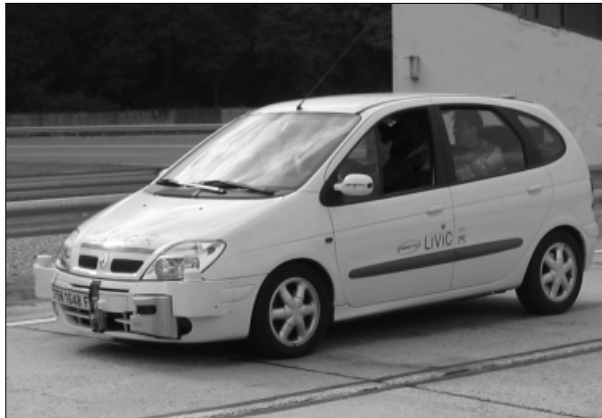
Fig. 10. The prototype vehicle, equipped with stereovision sensor, laser scanner sensor, odometer, inertial sensor, and automatic braking system.
