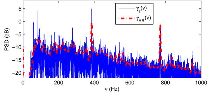
**Fig. 4:** Power spectral density of a real radiated noise of ship [7] and its 100<sup>th</sup> order autoregressive model.
