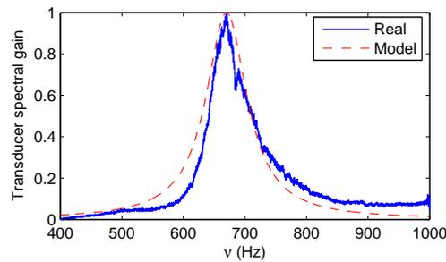
**Fig. 2:** Comparison between the spectral gain of the real transducer and the frequency resonator model (with  $\nu_r=667$  Hz et  $a=253.5$  estimated by the least square fitting method).
