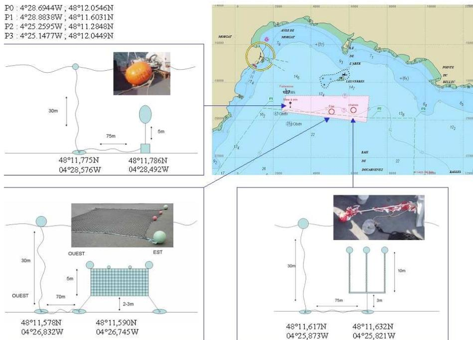
Figure 2: objects laid in The Bay of Douarnenez for the DEVITOBS’06 trial
