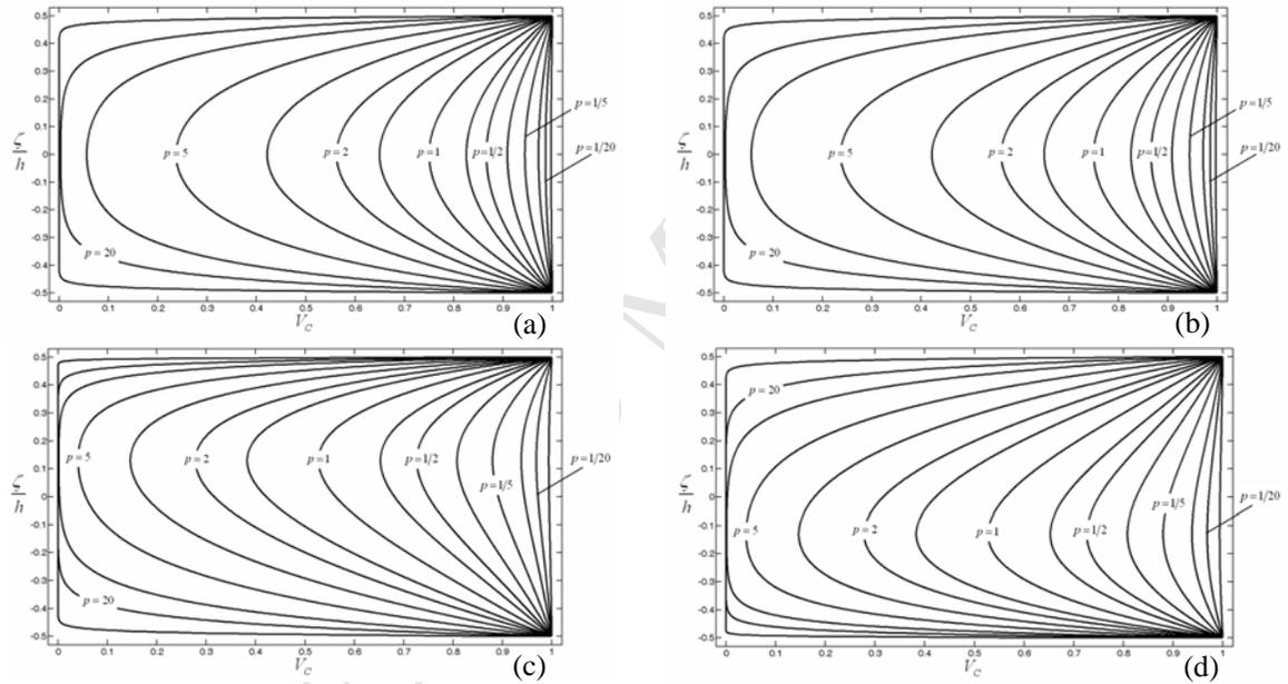
Figure 4. Variations of the ceramic volume fraction  $V_c$  through the thickness for different values of the power-law index  $p$ : (a)  $FGM_{1(a=1/b=1/c=2/p)}$ , (b)  $FGM_{2(a=1/b=1/c=2/p)}$ , (c)  $FGM_{1(a=1/b=1/c=4/p)}$ , (d)  $FGM_{2(a=1/b=1/c=4/p)}$ .
