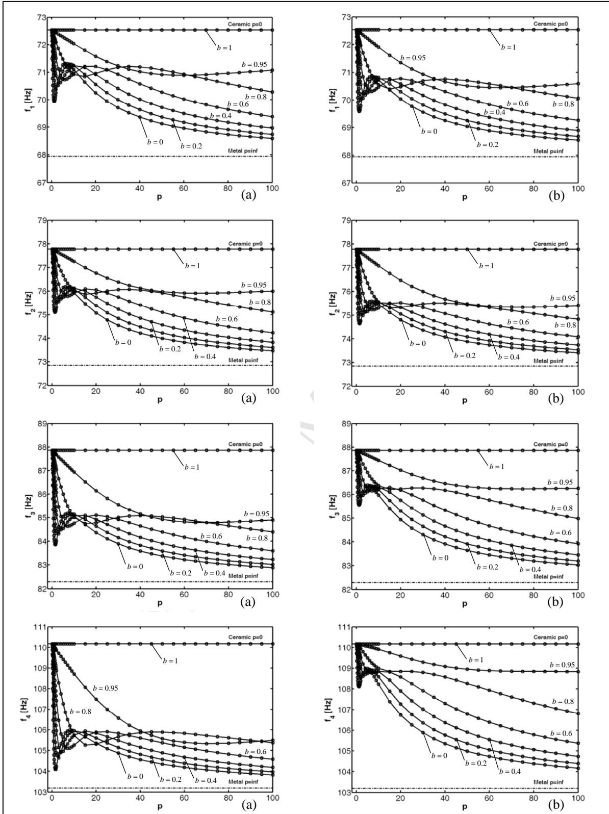
Figure 12. The first four frequencies of functionally graded toro-parabolic panel (S-F-S-F) versus the power-law exponent  $p$  for various values of the parameter  $b$  : (a)  $FGM_{1(a=1/0 \leq b \leq 1/c=1/p)}$ , (b)  $FGM_{2(a=1/0 \leq b \leq 1/c=1/p)}$ .
