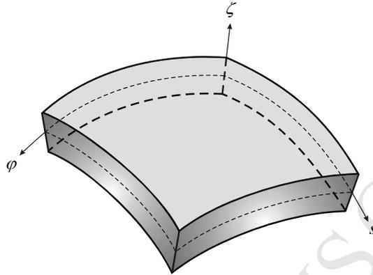
Figure 1. Co-ordinate system of doubly curved shell.
