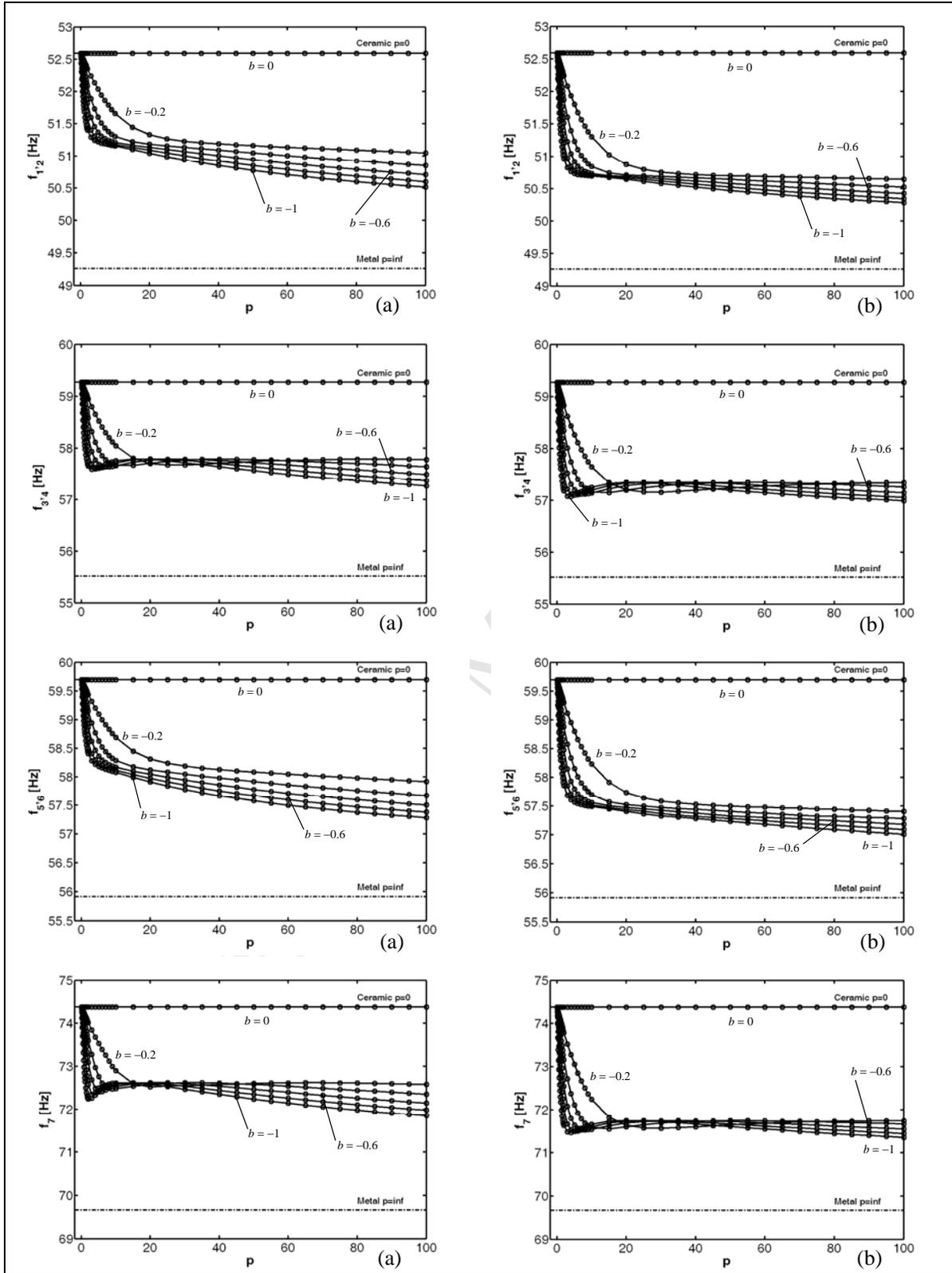
Figure 14. The first four frequencies of functionally graded parabolic toroid (F-C) versus the power-law exponent  $p$  for various values of the parameter  $b$  : (a)  $FGM_1(a=0/-1 \leq b \leq 0/c=2/p)$ , (b)  $FGM_2(a=0/-1 \leq b \leq 0/c=2/p)$ .
