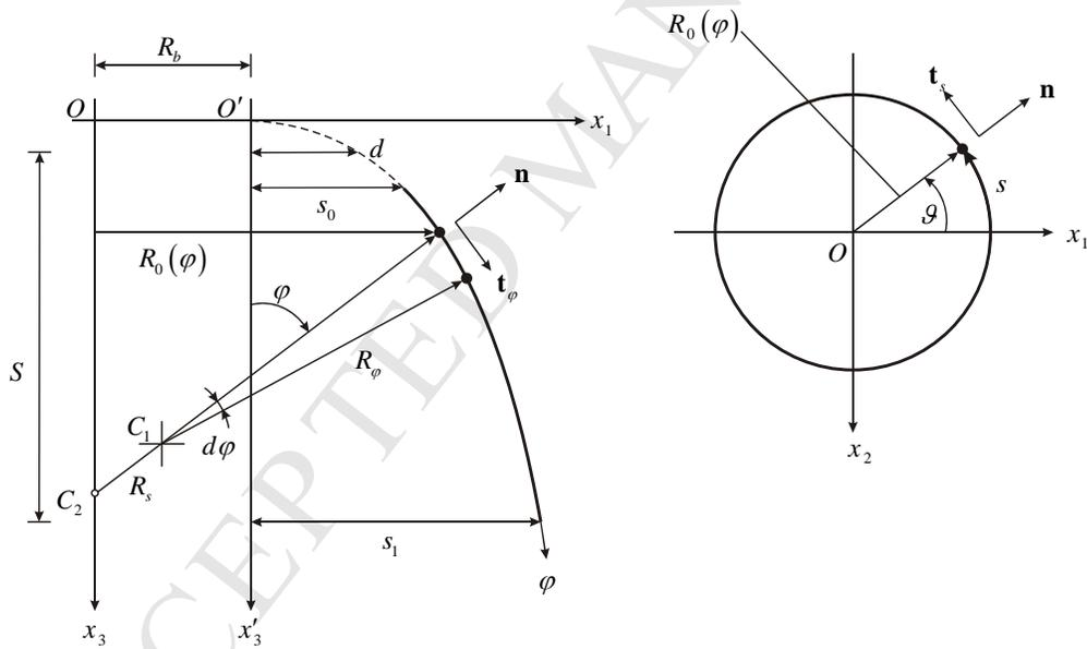
Figure 2. Shell geometry.
