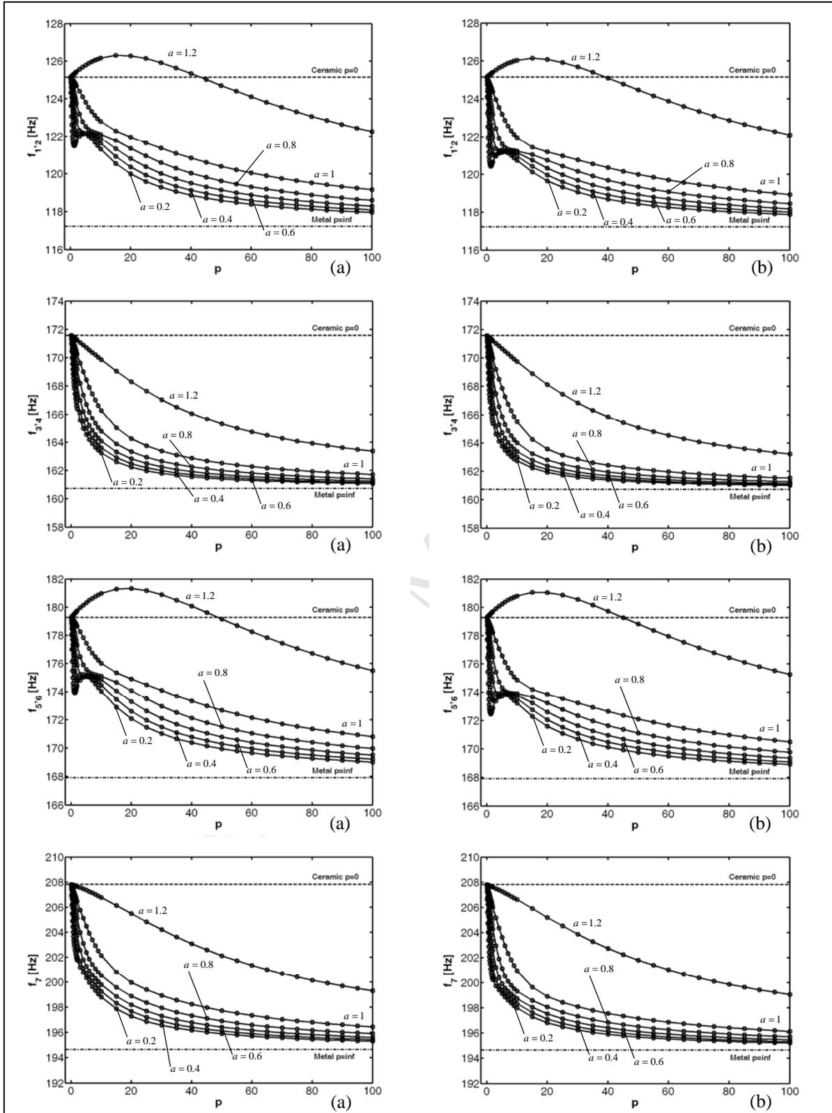
Figure 15. The first four frequencies of functionally graded parabolic dome (C-F) versus the power-law exponent  $p$  for various values of the parameter  $a$  : (a)  $FGM_1(0.2 \leq a \leq 1.2/b=0.2/c=3/p)$ , (b)  $FGM_2(0.2 \leq a \leq 1.2/b=0.2/c=3/p)$ .
