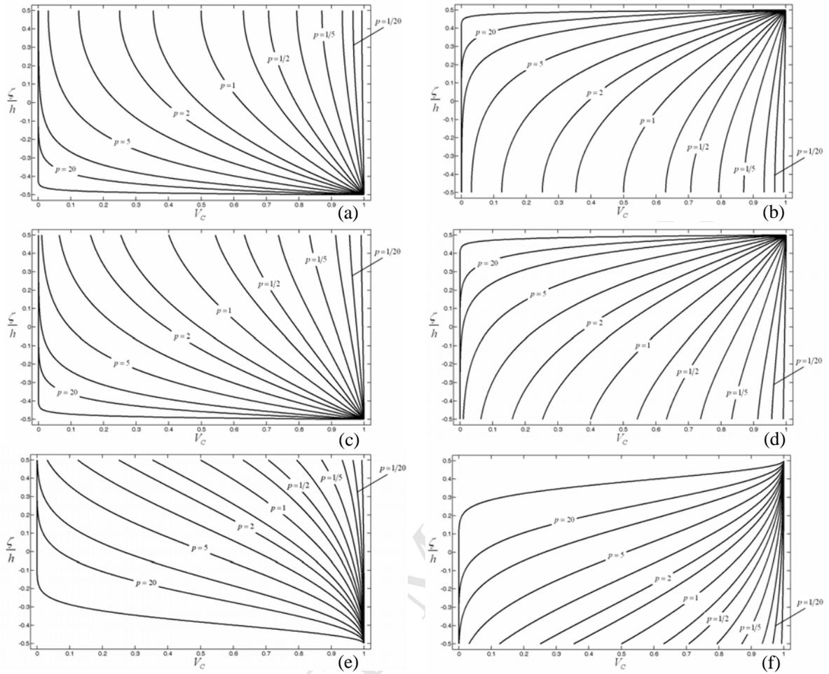
Figure 5. Variations of the ceramic volume fraction  $V_c$  through the thickness for different values of the three parameters  $a, b, c$  and the power-law index  $p$ : (a)  $FGM_{1(a=1/b=0.5/c=2/p)}$ , (b)  $FGM_{2(a=1/b=0.5/c=2/p)}$ , (c)  $FGM_{1(a=0.8/b=0.2/c=3/p)}$ , (d)  $FGM_{2(a=0.8/b=0.2/c=3/p)}$ , (e)  $FGM_{1(a=0/b=0.5/c=2/p)}$ , (f)  $FGM_{2(a=0/b=0.5/c=2/p)}$ .
