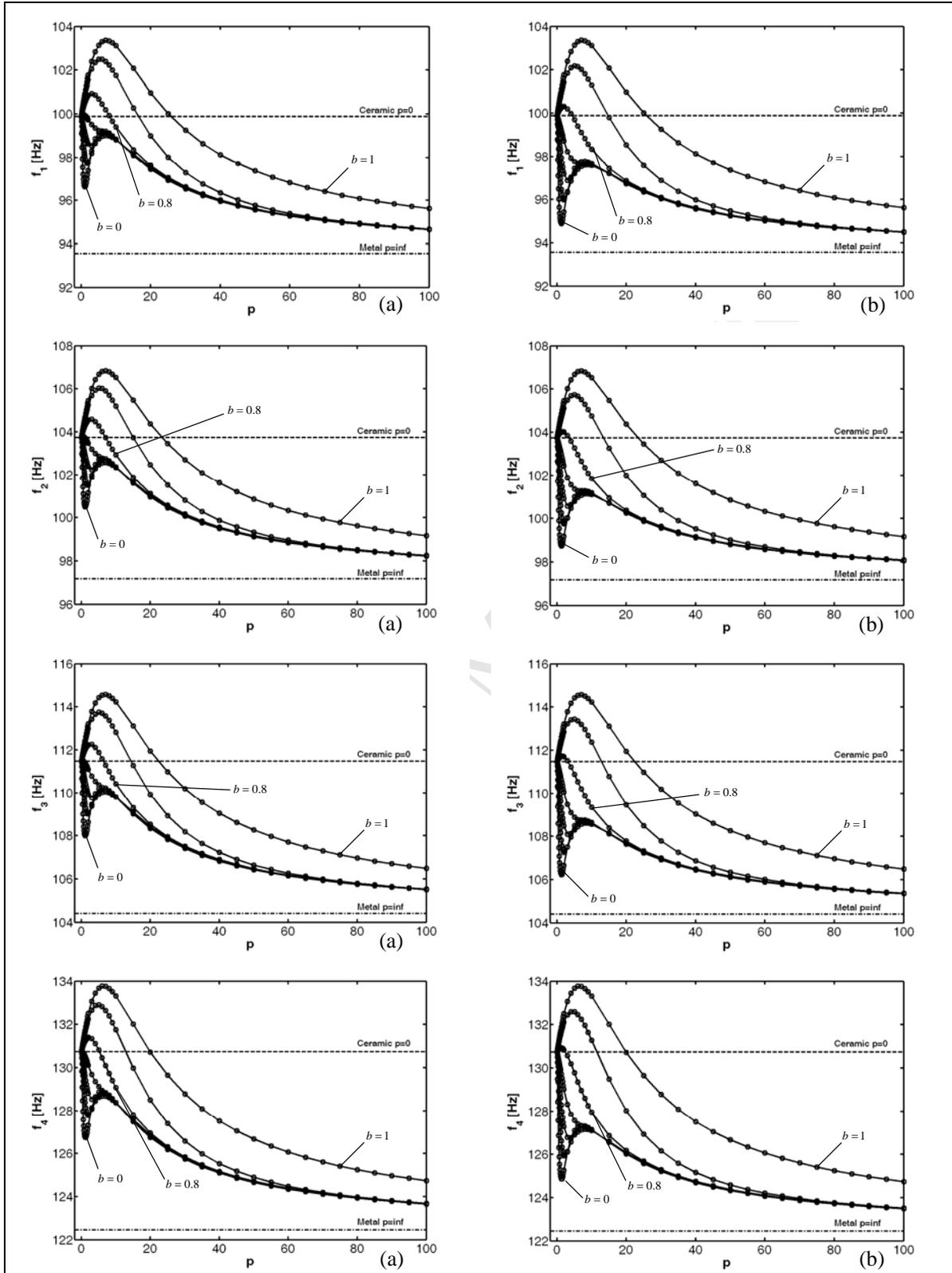
Figure 11. The first four frequencies of functionally graded toro-parabolic panel (C-F-C-F) versus the power-law exponent  $p$  for various values of the parameter  $b$  : (a)  $FGM_1$  ( $a=1/0 \leq b \leq 1/c=2/p$ ), (b)  $FGM_2$  ( $a=1/0 \leq b \leq 1/c=2/p$ ).
