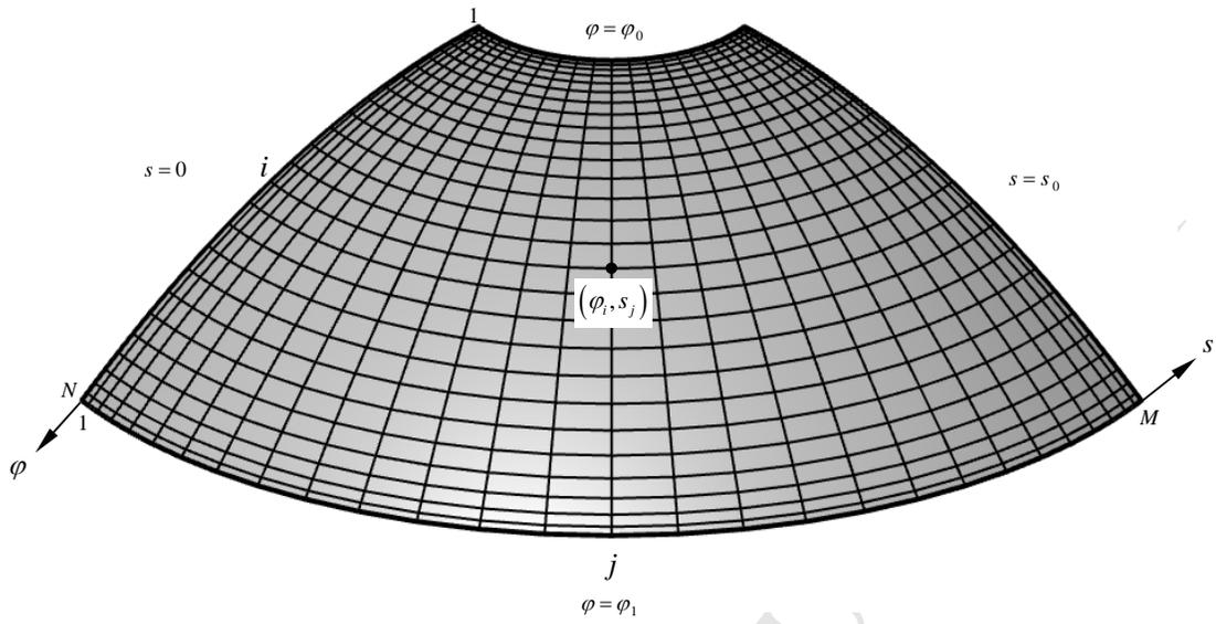
Figure 6. C-G-L grid distribution on a parabolic panel.
