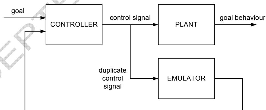
Fig.3. Architecture of a pseudo-closed loop control system (after Grush, 2004).
