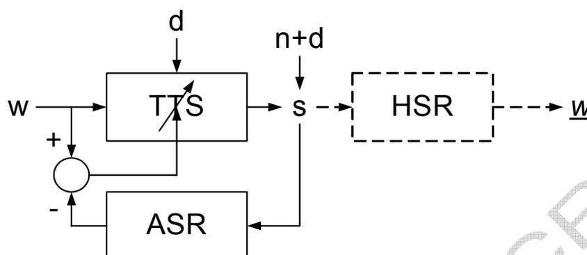
Fig.7. PRESENCE-inspired architecture for a novel form of text ( $w$ ) to speech ( $s$ ) synthesiser which alters its output in order to maximise recognition accuracy in the listener in response to arbitrary noise ( $n$ ) and disturbance ( $d$ ).
