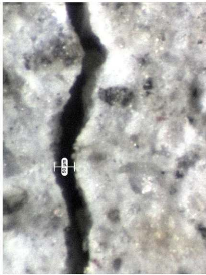
c) \text{COD}_{\text{max}} = 154 \text{ } \mu\text{m} , w_1 \approx 50 \text{ } \mu\text{m}
