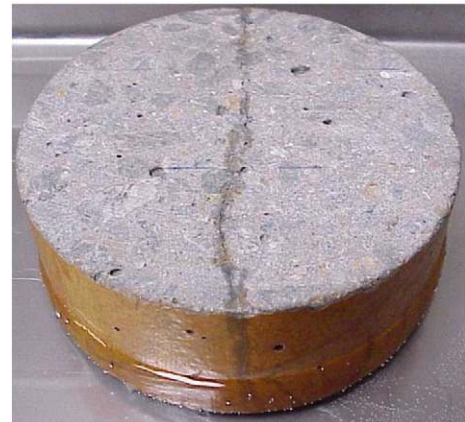
Fig. 12. Wetted zone around the main crack on the upper face of HPC disc during imbibition.
