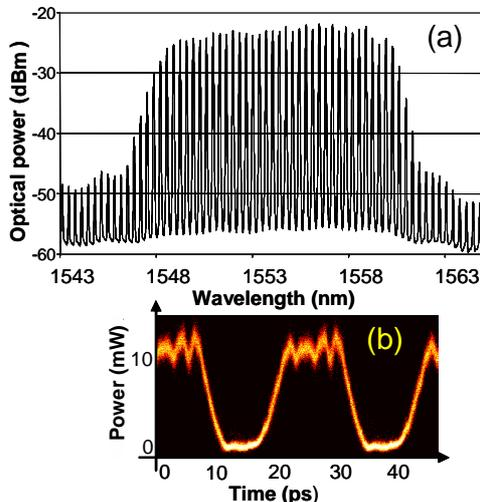
Fig. 1: Optical spectrum and corresponding eye diagram.
