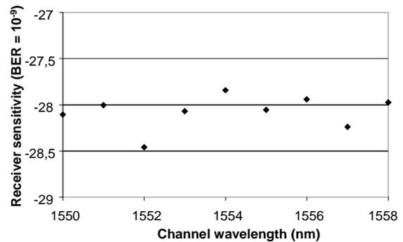
Fig. 6: Receiver sensitivity measurements at BER = 10<sup>-9</sup>.
