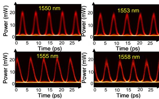
Fig. 3: 170 Gbit/s eye diagrams at 4 wavelengths.
