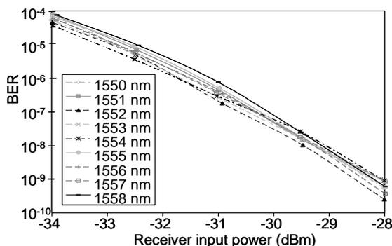
Fig. 5: BER measurements on a 9 nm bandwidth.
