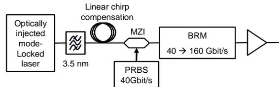
Fig. 2: Transmitter setup
