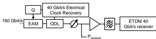
Fig. 4: Receiver setup.
