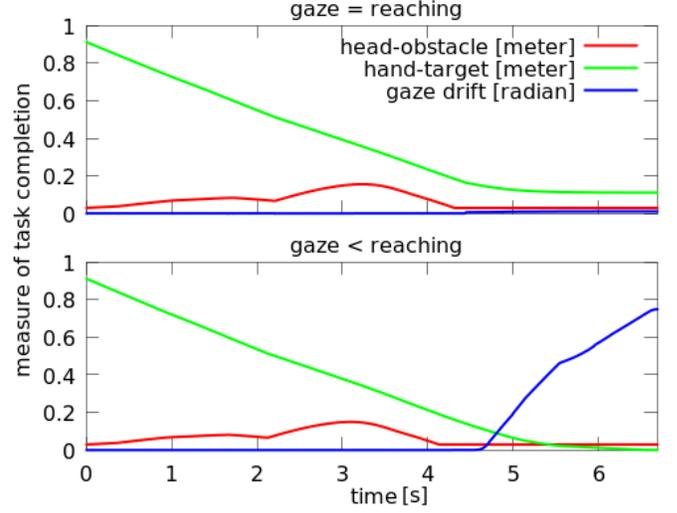
Fig. 6. Effect of prioritization in Scenario 1. Upper window: a single priority stage is used to solve the *reaching* and *gaze* under constraints: neither of the tasks is completed. Lower window: the *gaze* task placed in priority 2 diverges to the benefit of reaching for the target point (priority 1).
