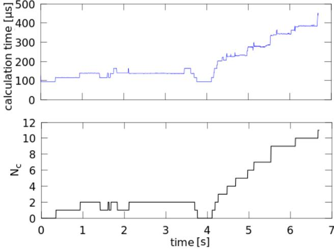
Fig. 7. Scenario 1. Upper window: cost of preparing and solving the sequence of prioritized linear systems per time step. Lower window: number  $N_c$  of saturated inequality constraints per time step. Every iteration counted 33 inequality constraints for collision avoidance and 56 for lower and upper bounds. The program was run in a single thread using the notebook processor Intel Core i5-540M at 2.52 GHz.
