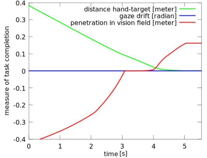
Fig. 9. Effect of prioritization in Scenario 2. The inequality task responsible for keeping the center of the hand (point  $p_h$ ) out of the vision field holds until becoming conflicting with the higher-priority reaching task.
