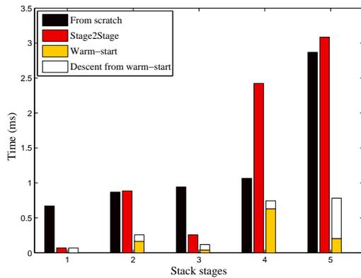
Fig. 1. Computation cost (in ms) for the set of five QPs alone (*from scratch*), the five QPs using at each stage  $N+1$  the result of stage  $N$  for initialization (*stage2stage*), and using warm start (this last one being divided in two cost, for warm start and for the QP itself).
