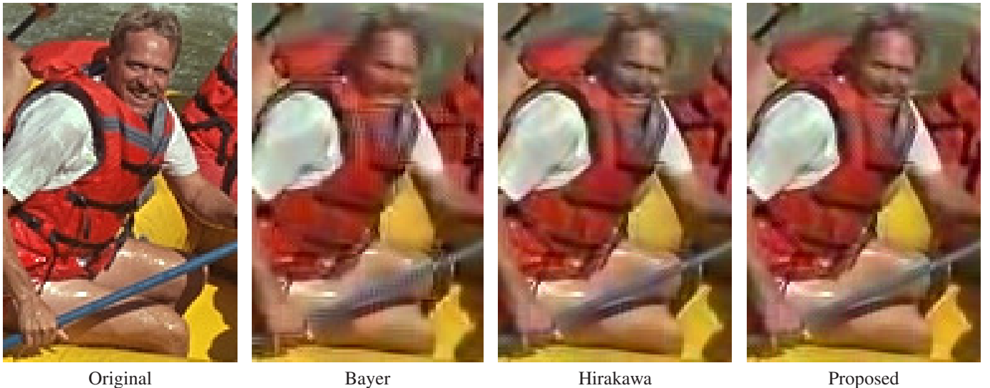
Fig. 7. Results of joint demosaicking and denoising, as described in Sect. IV-C, with the three CFAs depicted in Fig. 1, on a part of the Kodak image no. 14. The mosaicked image were corrupted by additive white Gaussian noise of standard deviation \sigma = 40 and the BM3D denoising method was used.
