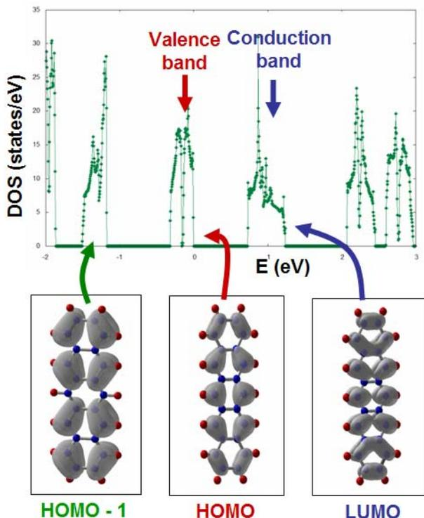
**Fig. 1.** Band formation in a pentacene crystal: (top) electronic density of states of pentacene, and (bottom) amplitudes of the respective highest occupied (HOMO) and lowest unoccupied (LUMO) orbitals of pentacene. The orbital below the HOMO (HOMO-1) is also shown.
