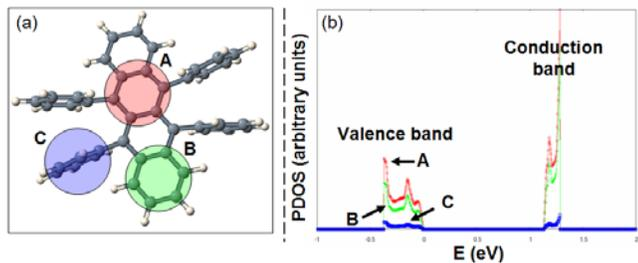
**Fig. 3.** Contribution of the encircled C rings of (a) in the electronic density of states (b) of rubrene. The tetracene backbone of rubrene has an enhanced role in the formation of the valence and conduction bands.
