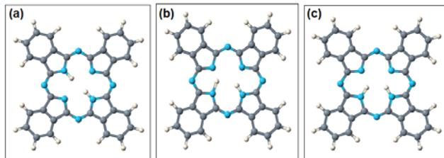
**Fig. 5.** Transformation of metal-free phthalocyanine (Pc) with 2 H atoms at the Pc core: (a) and (c) are initial and final configurations, (b) is the transition state. The DFT-GGA energies of (b) and (c) are larger than that of (a) by 0.49 eV and 0.34 eV, respectively.
