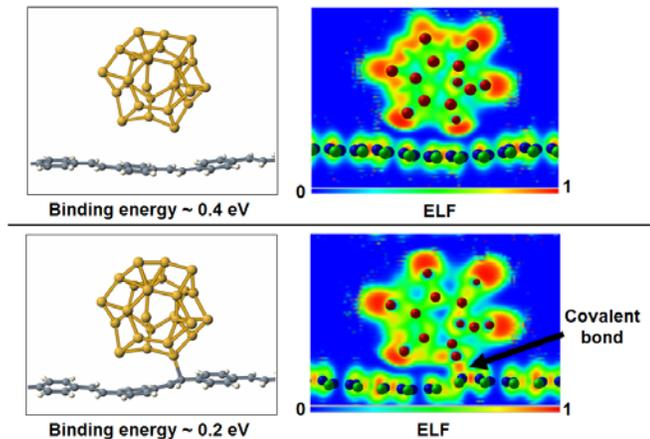
**Fig. 4.** Stable configurations of the hybrid system of a Si cluster with 27 atoms and a PPV chain. The images on the right are contour plots of the electron localization function (ELF), showing the formation of a covalent bond between the Si cluster and the PPV chain in the second case.
