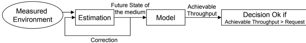
Fig. 3. Design of the admission control algorithm for EDCA
