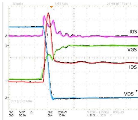
Fig. 9. Measurement at Turn-On. U=270V , I=8A . The experimental test bench is described in figure 5.
