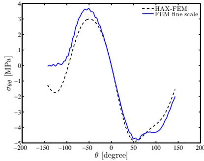
Figure 4: Comparison of hoop stress distribution along a circle of radius  $d$  (the width of the notch) obtained with HAX-FEM and a fine FE model for a combined tension / shear (10 kN) load at initiation.
