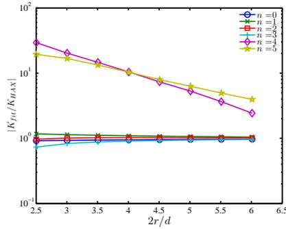
Figure 5: Ratio between Williams' coefficients obtained by least-squares fit of the fine FE results and those obtained with HAX-FEM for a combined tension / shear loading at initiation. Only mode  $I$  coefficients are plotted as functions of normalized size of the domain used for the least-squares fit.
