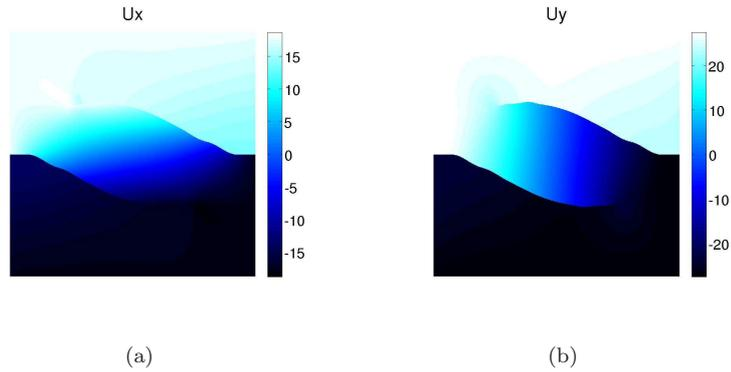
Figure 6: Horizontal (a) and vertical (b) displacement (in  $\mu\text{m}$ ) during crack propagation for a shear preload of 10 kN.
