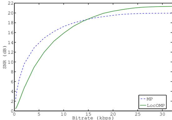
**Fig. 2.** SNR depending on the decoding bit rate
