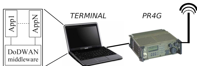
Figure 5. Architecture of a typical mobile unit running DoDWAN
