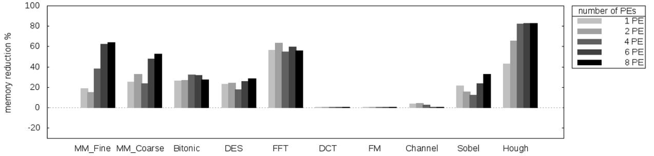
Fig. 6. Minimal required memory reductions achieved by our proposed method: the results are expressed as a reduction percentage over the minimal required memory per PE obtained by *MPA-ii* in [5]
