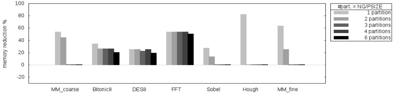
Fig. 7. Evaluation of the partitioning heuristic on 8 PE: for each benchmark, we show the memory reduction achieved when changing  $\frac{N_G}{P_{SIZE}}$  (the number of partitions used), exhaustive search is conducted independently in each partition.
