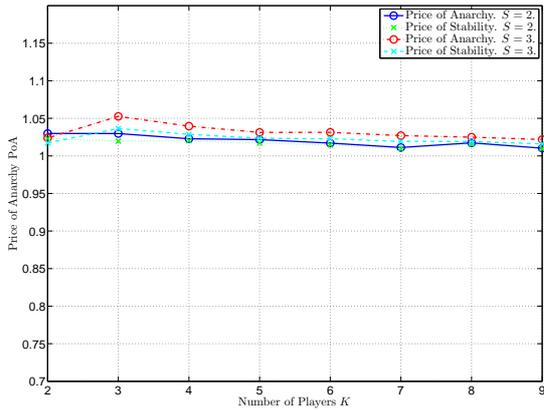
**Figure 5: Price of anarchy (Def. 10) and price of stability (Def. 10) as a function of the number of players  $K$  for the case of two and three BSs,  $S = 2$  and  $S = 3$ .  $SNR = 10 \log_{10} \left( \frac{p_{\max}}{N_0 B} \right) = 10$  dB.**
