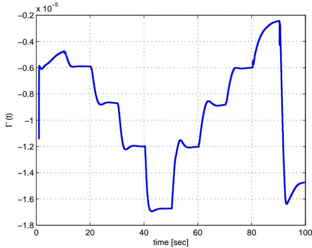
Fig. 6.  $\Gamma(t)$  during a transient load at 1500 rpm when a leakage hole of 4mm is present
