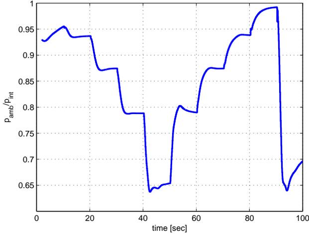
Fig. 3. Pressure ratio  $p_{amb}/p_{int}$  during a transient load at 1500 rpm.
