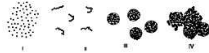
Figure 1: Schematic representation of the steps of multiscale agglomeration according to Refs 8 and 9
