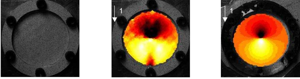
**Figure 2.** Quasi-static test, (a) raw image of the specimen before the test, (b) 1\_displacement field computed for a test on the shell TP-composite, (c) 1\_displacement field computed for a test on aluminium sheet.
