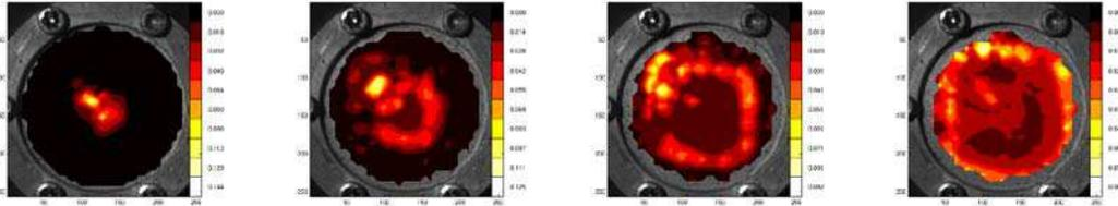
**Figure 3.** Visualisation of the propagation of the flexural wave during a dynamic perforation test ( $dt=35 \mu s$ )
