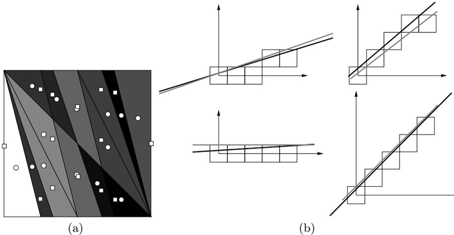
**Fig. 4.** Comparison between the proposed representative straight line computation (circles in (a) and bold lines (b)) and the existing approach (squares in (a) and gray lines in (b)): (a) differences depicted in the Farey Fan of order 4 and (b) in the primal space.
