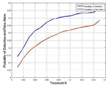
**Fig. 3.** PHAD : Probability of Detection ( $PD$ ) and Probability False Alarm ( $PF$ ) vs. threshold parameter  $k$ ,  $PD = f(k)$  and  $PF = g(k)$ .
