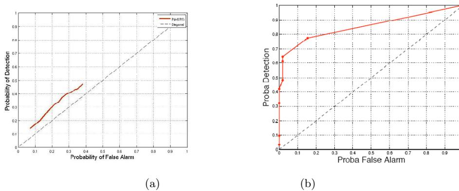
**Fig. 2.** Statistical performances of (a) PHAD and (b) Gamma-FARIMA approach evaluated thanks to the METROSEC database. Detection Probability ( $PD$ ) vs. Probability of false alarms ( $PF$ ),  $PD = f(PF)$ .
