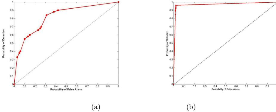
**Fig. 1.** Statistical performances of NADA evaluated based on (a) the MetroSec database and (b) the 10% KDD database. Detection Probability ( $PD$ ) vs. Probability of false alarms ( $PF$ ),  $PD = f(PF)$ .
