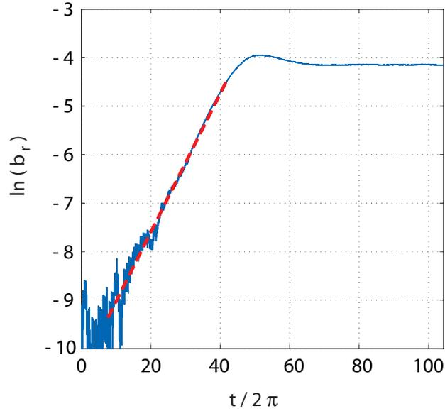
Figure 4: Logarithm of the induced magnetic field signal (full line) at  $E = 8.53 \times 10^{-5}$ ,  $\epsilon = 0.100 \pm 0.005$ ,  $\Lambda = 0.01$ . The slope of the linear fit (dashed line) provides the initial linear growth rate.
