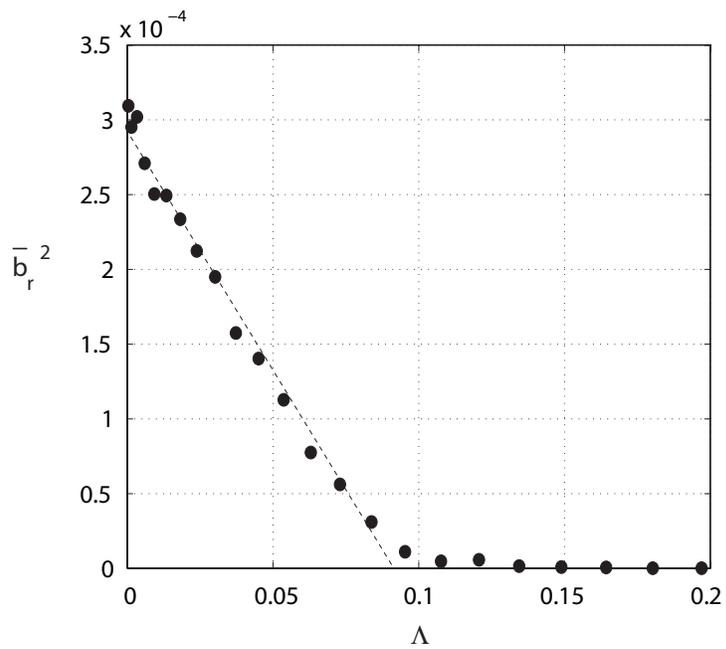
Figure 6: Square of the measured saturation-amplitudes of the magnetic field  $b_{r, sat}^2$ , as a function of Elsasser number  $\Lambda$ .  $E = 8.5 \times 10^{-5}$ ,  $\epsilon = 0.10$ . Experimental measurements ( $\bullet$ ) and linear fit (dashed line). The saturation amplitudes are in agreement with the weakly nonlinear scaling, predicting a linear dependence on  $\Lambda$ .
