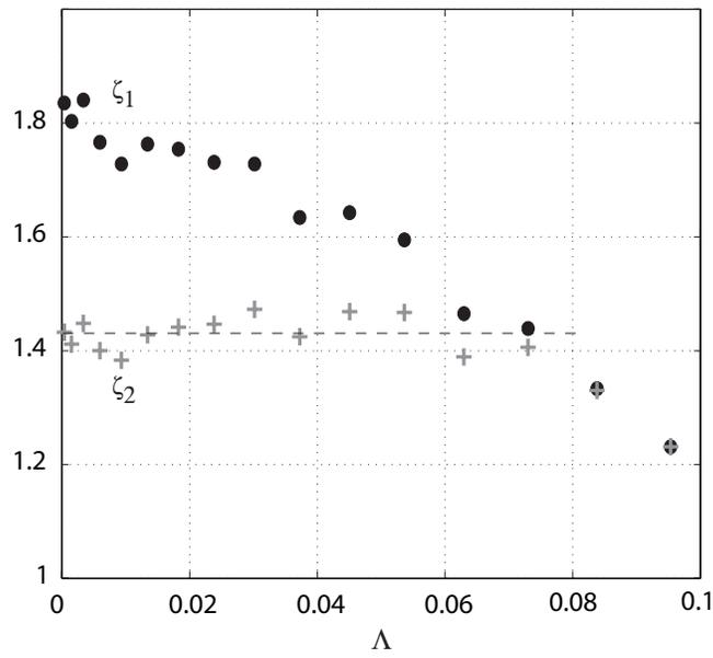
Figure 7: Ratios of the experimentally observed saturation amplitude, to the theoretical saturation amplitudes  $\zeta_1$  (●) and to the maximum amplitude attained during the overshoot  $\zeta_2$  (+), as a function of the Elsasser number  $\Lambda$ .  $E = 8.5 \times 10^{-5}$ ,  $\epsilon = 0.10$ .
