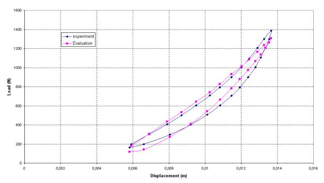
Figure 3 Example of testing results for the determination of shoe mechanical parameters.
