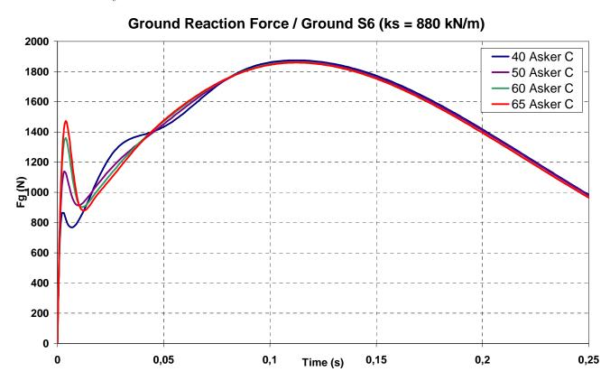
Figure 5 Ground reaction force  $F_g$  for soil S6 (Ground stiffness: 880 kN/m).
