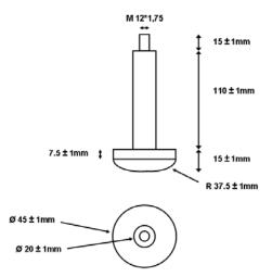
Figure 2 The indenter used for loading the shoe sole and the characterization of mechanical parameters.
