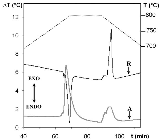
Fig. 8. Thermal behaviour upon first cycle of two cold-pressed powder mixtures analysed by SDTA at 4 °C.min<sup>-1</sup>: mixture R with composition Ag:Cu = 60:40 at% and mixture A with composition Ag:Cu:Ti = 43:28.5:28.5 at% (temperature versus time is drawn in the upper part of the graph)
