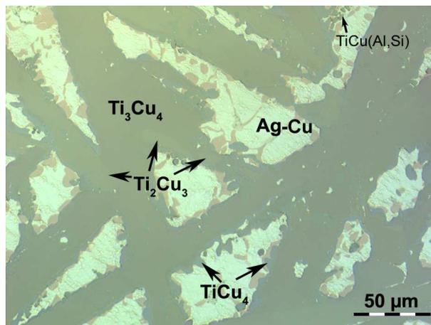
Fig. 5.  $\text{Ti}_3\text{Cu}_4$  plate-like crystals grown in mixture F first reacted at 825 °C for 353 h and then annealed at 854 °C for 50 min (note the difference with Fig. 3)
