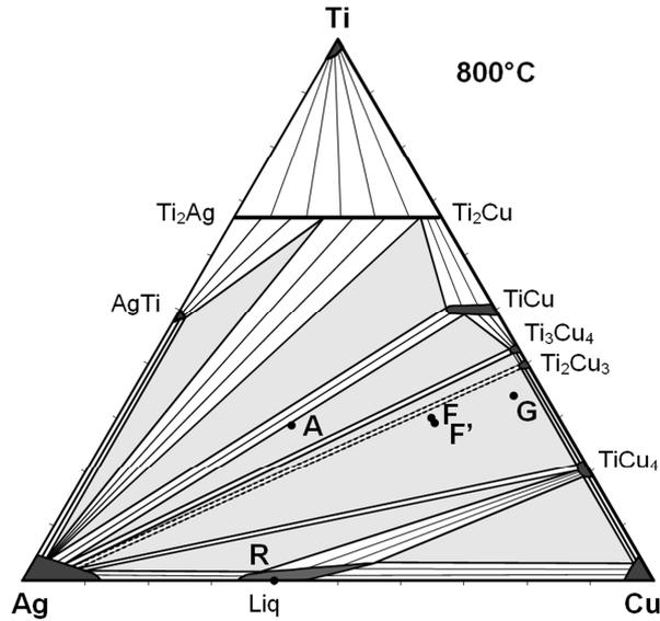
Fig. 1. Ag-Cu-Ti isothermal section at 800 °C, according to experimental data and thermodynamic evaluations [6-16]. The tie lines joining  $Ag_s$  to  $Ti_2Cu_3$  have been drawn in dotted lines since for Eremenko et al. [6-8],  $Ti_2Cu_3$  is not stable at 800 °C
