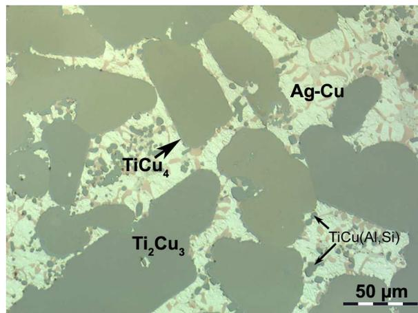
Fig. 3.  $\text{Ti}_2\text{Cu}_3$  globular crystals in a silver-rich matrix, as synthesized in mixture F after heating at 825 °C for 353 h: small crystals in the matrix analyse for  $\text{TiCu}(\text{Al},\text{Si})$  whereas  $\text{TiCu}_4$  crystals are stuck onto  $\text{Ti}_2\text{Cu}_3$
