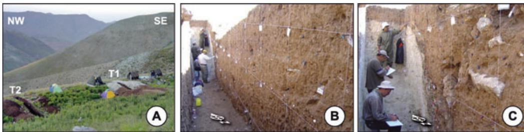
Figure 10. (a) Field picture showing the trenches T1 and T2 dug across the fault scarp, immediately west of the topographic survey shown in Fig. 8. (b) Northward view of trench T1. (c) Close-up of the fault zone within the eastern wall of the trench T1.
