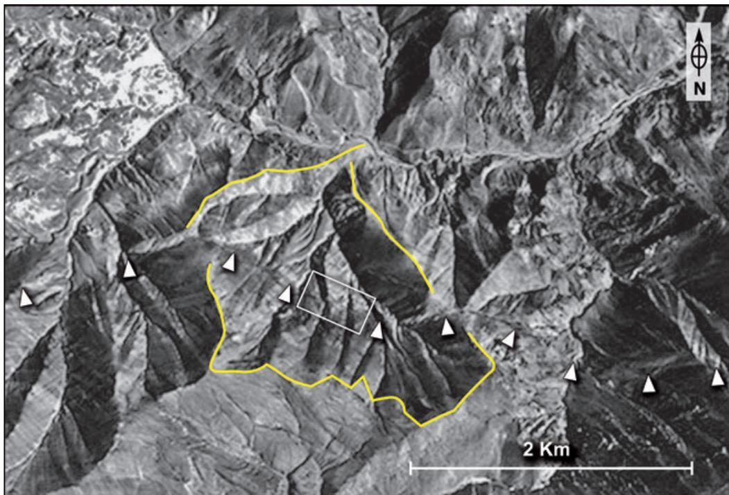
**Figure 7.** Aerial photo of the active Taleghan fault in its eastern part showing the left-lateral normal displacement of a drainage basin (yellow line), its crests and talwegs (see Fig. 3 for location). White triangles indicate the fault line. The white rectangle indicates the area studied in details.
