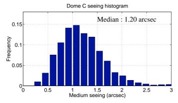
**Fig. 1.** Normalized histogram of seeing for an exposure time of 10 ms. Transversal and longitudinal values have been averaged.
