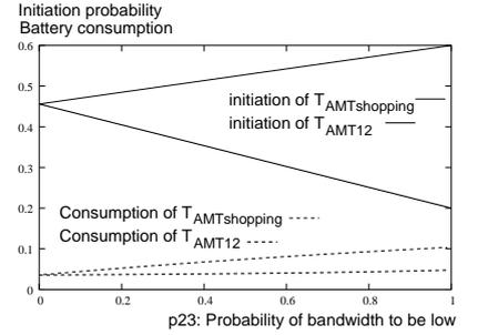
Figure 4: Initiation probability and battery consumption vs bandwidth.
