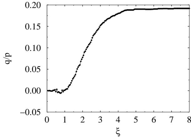
**Figure 5.** The partial shear stress, normalized by the mean stress, as a function of force threshold  $\xi$ .
