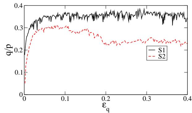
**Figure 9.** Normalized shear stress  $q/p$  as a function of cumulative shear strain for the samples S1 and S2.
