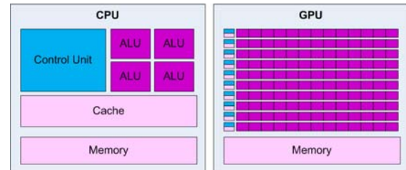
Figure 4: Comparison of the architecture of CPU and GPU.
