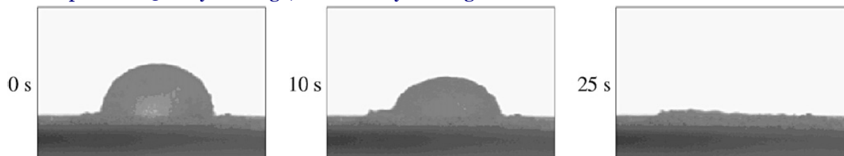
Fig 20: Evolution of the water drop after 36 days storage under constant RH: 33%.
