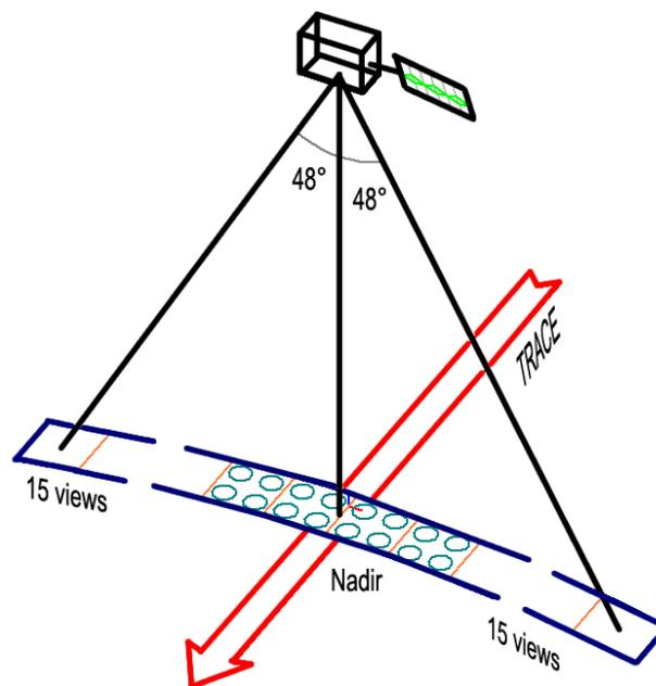
**Fig. 1.** IASI observing mode: the instrument measures the spectrum of infrared radiation emitted by the Earth and the atmosphere, from a low altitude sun-synchronous orbit, over a swath width of ~2200 km, every 50 km at nadir (with 4 footprints of 12 km in diameter).
