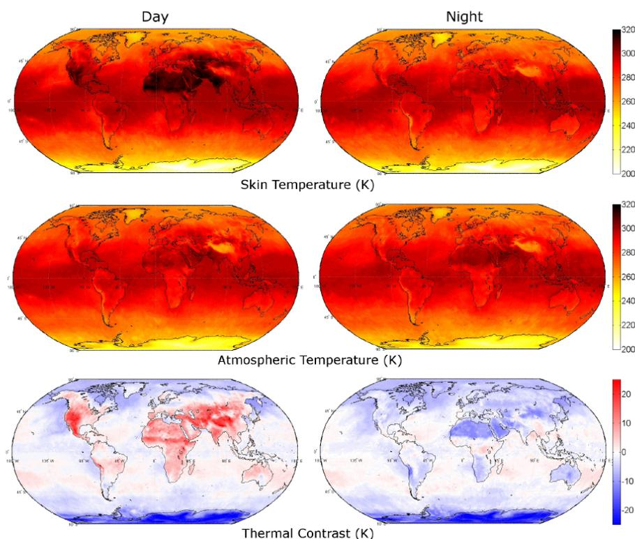
**Fig. 7.** Upper and middle panels represent skin temperatures and the first level of retrieved temperatures available from Eumetsat Level 2 products, for daytime (left) and nighttime (right) observations, averaged over May 2008. The bottom plots are the difference between these temperatures (thermal contrast).
