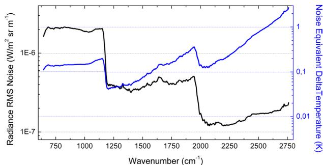
**Fig. 2.** IASI radiometric noise as established from a set of representative spectra, spanning a range of latitude. Values are provided in radiance units (W/(m<sup>2</sup> sr m<sup>-1</sup>), black line, left scale), and were converted to noise equivalent temperature difference (Ne $\Delta T$ , blue line, right scale) for a given reference temperature of 280 K.
