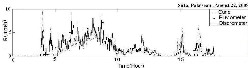
**Figure 6:** Comparison of Rainfall Rate  $R$  (mm/h) between CURIE at 60 m, the LATMOS disdrometer, and the rain gauge as a function of time (local precipitation) during precipitation at SIRT A on August 22, 2008.
