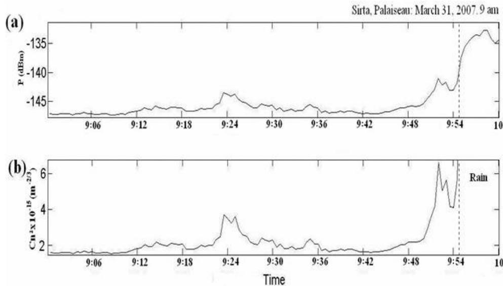
**Figure 2:** Response of CURIE in clear air at an altitude of 130 m, (a) Received Power  $P$  in dBm as a function of time, (b) Equivalent  $C_n^2$  ( $\times 10^{-15} m^{-2/3}$ ) as a function of time; SIRTA on March 31, 2007; local time.
