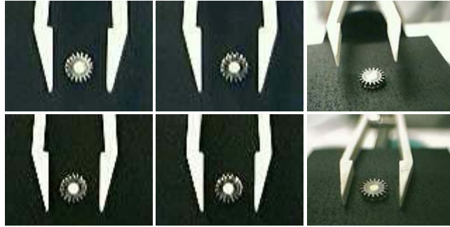
Fig. 9. Top, stereo top images and lateral image of the scene with the microgear outside the gripper tips. Bottom, the same scene with the microgear inside the gripper tips.
