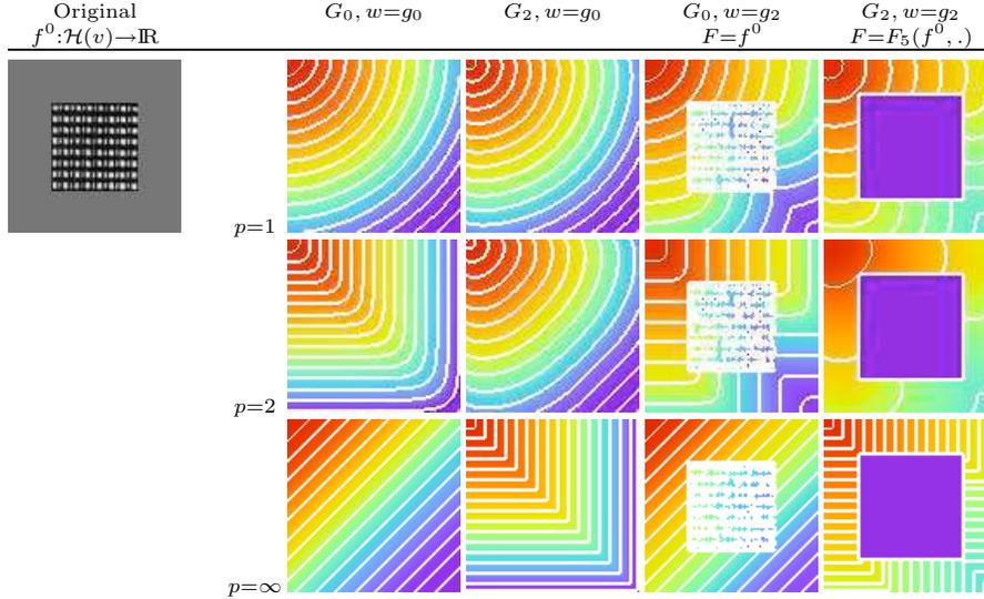
**Fig. 1.** Front propagation and weighted distances with different  $p$  values, graph configurations  $G$ , weights  $w$  and features  $F$ . Figures represent color distance maps with iso-level sets obtained by thresholding the distances. The seed is located at the top left corner (see text for more details).
