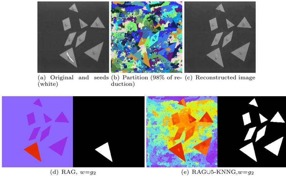
**Fig. 3.** Nonlocal region based image segmentation. (a) original image ( $256 \times 256$ ) with 65 536 pixels. (b) partition with 1 324 regions (98% of reduction as compared to original one). (d) and (e) at left, distance color maps (red for small and blue for large distances) and at right, final segmentations. Graphs used in (d) and (e) are computed from (b) and (c) (see text for more details).
