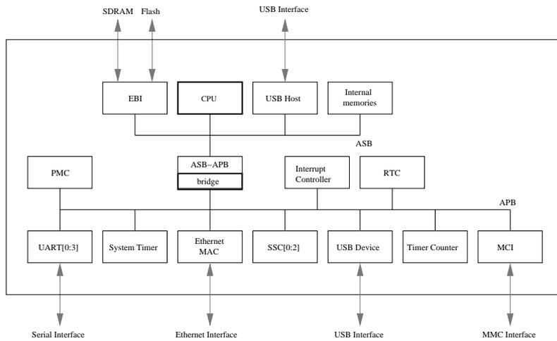
Figure 10: AT91RM9200 architecture. Bold blocks are bus masters
