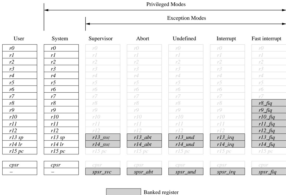
Figure 3: Banked registers of ARM CPU
