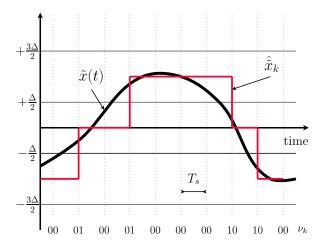
Fig. 2. Illustration of the level detector working operation principe.
