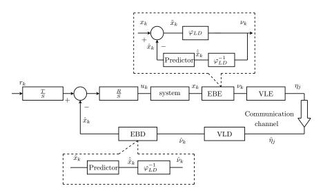
Fig. 1. Block diagram of the non uniform entropy coding in the feedback loop.
